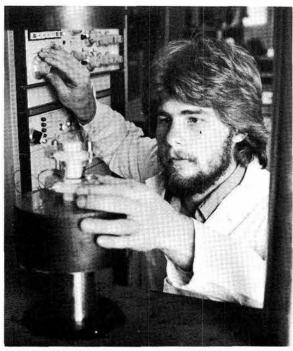
JERRY O'BRIEN adjusts rock sample for a uniaxial compression test to measure stress/strain response.
